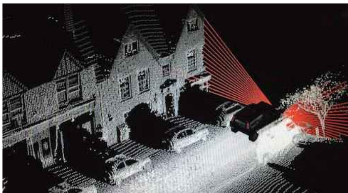
Autonomous car uses a laser scanner to build a 3D map of the surroundings
